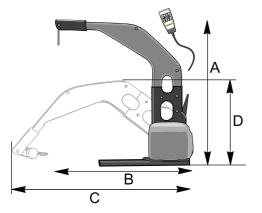
A= 105 cm including mounting base. The hoist is height adjusted by cutting (down to 74 cm).
