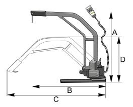
A= 106 cm including mounting base. Height adjusted by cutting. B= 109 cm. Length adjusted by cutting. C= Max 141 cm folded D= Max 58 cm
