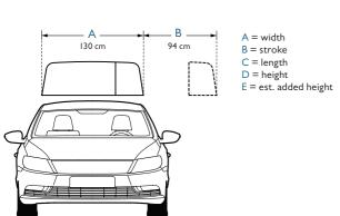
The Chair Topper stores a foldable wheelchair within 30 seconds. The weather-tight fibreglass compartment weighs 55 kg and can be mounted on most vehicle models. The total weight, including wheelchair, does not exceed 75 kg.
